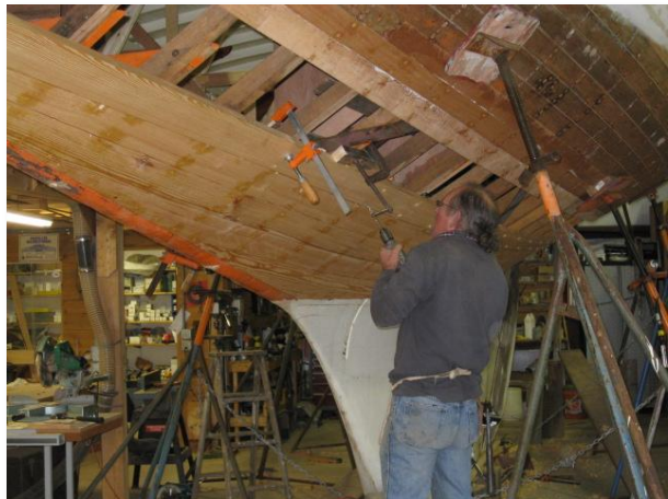
Figure 24 - Port Planking. (Courtesy Wayne George).
