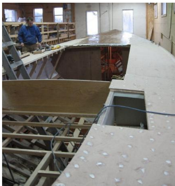
Figure 17 - Deck Completion. (Courtesy Doug Hylan).
